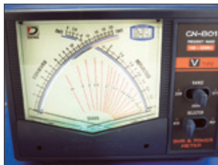
Figure 1 — The Daiwa CN-801 SWR/power meter is a versatile instrument. The meter face is illuminated by a small bulb below the bottom of the meter movement.
